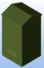
FDMS 650 Front and Rear Access Cabinets are designed for external use, manufactured from 2mm thick 4003 stainless, the fully welded Construction ensures the Cabinets are robust and suitable for heavy-duty applications.
