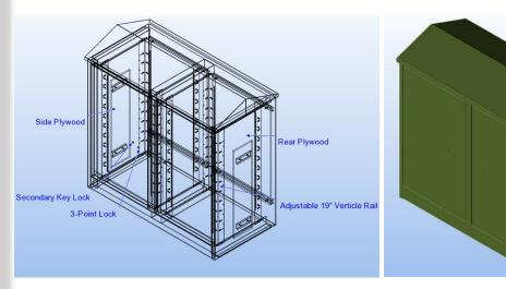
FDMS 650 double bay Front Access Cabinets are designed for external use, manufactured from 2mm thick 4003 stainless, the fully welded Construction ensures the Cabinets are robust and suitable for heavy-duty applications.
